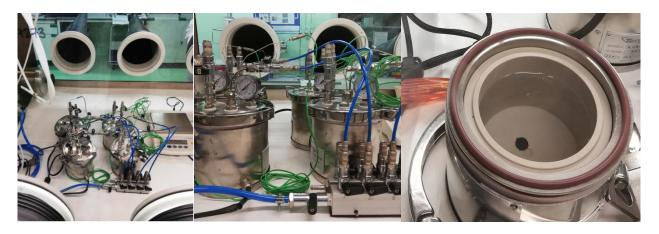
Figure 2.1.4.1.- View of leaching experimental set up installed at CIEMAT in Ar glove box under 8 bar of 4.7%  $H_2$ - $N_2$ .
