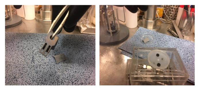
Figure 2.2.1.1: View of the samples (MOX pellets and iron foil) at the end of the leaching experiment.
