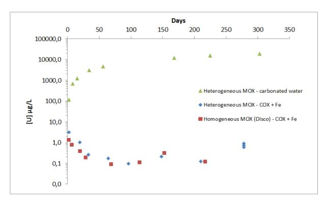
Figure 2.2.1.3: Evolution of the uranium concentrations as a function of time in a carbonated water for an heterogeneous Mimas MOX fuel (M Odorowski thesis) and for homogeneous and heterogeneous MOX fuels in a synthetic COX water + metallic iron.
