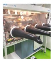
Figure 2.1.3.1 Experimental set-up under Ar glove box contitions. UO<sub>2</sub> fragments are placed into silica saucer and Fe strip leans to the wall of the polyethylene vessel.
