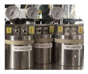
Figure 2.1.1.1: Stainless steel autoclaves
