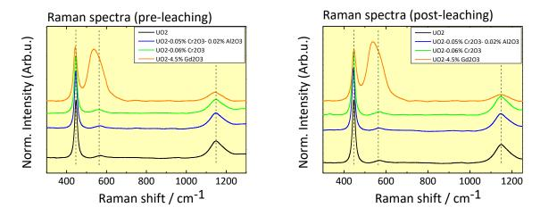
Figure 2.1.4.4.- Raman spectra of solid sample pre-leaching (a) and after 136 days of leaching time (b) for  $UO_2$ -0.06 $^{\rm w}$ / $_{\rm o}Cr_2O_3$ ,  $UO_2$ -0.05 $^{\rm w}$ / $_{\rm o}Cr_2O_3$ -0.02 $^{\rm w}$ / $_{\rm o}Al_2O_3$  and  $UO_2$ -4.5 $^{\rm w}$ / $_{\rm o}Gd_2O_3$  compared to  $UO_2$  spectra.
