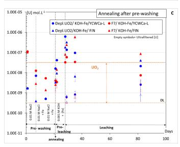
Figure 2.1.1.4: Third type of experiments - U concentration as function of time with depleted UO2 and F7 pellet as function of annealing, pre-washing with 0.01 M NaCl + (Fe) and pre-leaching with 0.001 M KOH+ (Fe) of the pellet at pH 13.5 in young cementitious water (YCWCa-L) and at pH 8.5 in bicarbonate water (FIN). A- experiments without annealing, no preleaching; B- annealing before pre-washing and pre-leaching; Cannealing after pre-washing and before pre-leaching.
