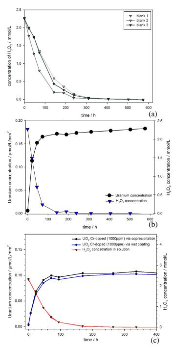
Figure 2.1.2.2: (a) Concentration of  $H_2O_2$  in exemplary blank runs without  $UO_2$  pellets. (b) Solution concentrations of U(VI) - normalised to the geometrical surface area of the pellet - and  $H_2O_2$  vs. time for an experiment using a pure  $UO_2$  pellet. (c) Solution concentrations of U(VI) - normalised to the geometrical surface area of the pellets - and  $H_2O_2$  in two experiments using Cr-doped pellets prepared via co-precipitation, and wet coating, respectively vs. time.
