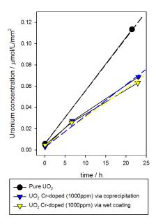
Figure 2.1.2.3: U(VI) concentrations in solution (normalised to the geometrical surface area of the pellets) during the first 24 hours of selected dissolution experiments, using a pure UO<sub>2</sub> reference (95 % relative density, black circles) and two representative Cr-doped UO<sub>2</sub> samples produced by co-precipitation (97.5 % relative density, blue triangles) and by wet coating (98.8 % relative density, yellow triangles).
