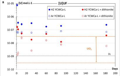
**Figure 2.1.1.2:** First type of experiments - U concentration as function of time with depleted  $UO_2$  pellet in autoclave experiments with and without 10 ppm dithionite ( $Na_2S_2O_4$ ) under Ar and  $H_2$  atmosphere at pH 8.5 in bicarbonate solution-FIN (A) and at pH 13.5 in young cementitious water (YCWCa-L) (B).
