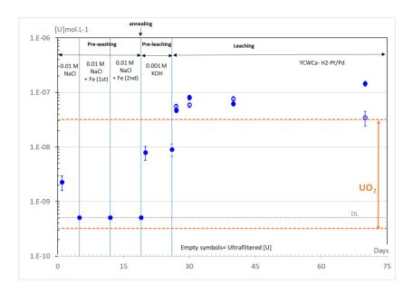
**Figure 2.1.1.3**: Second type of experiments - U concentration as function of time with depleted  $UO_2$  pellet for the autoclave experiment with Pt/Pd catalyst under  $H_2$  atmosphere at pH 13.5 in young cementitious water (YCWCa-L).
