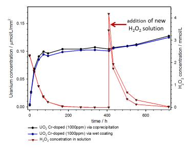
Figure 2.1.2.5: Concentrations of uranium and  $H_2O_2$  in solution depending on run time for two representative Cr-doped  $UO_2$  samples obtained by different doping methods.
