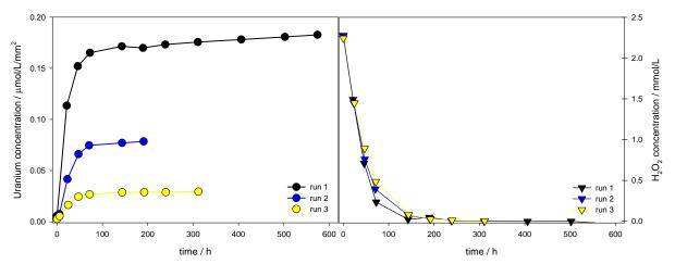
Figure 2.1.2.4: Concentration of uranium (left) and  $H_2O_2$  in solution (right) in repeated experiments using a representative reference sample (i.e pure  $UO_2$ ) as function of time. Between each run the pellet and the complete experimental setup was extensively washed with  $NaHCO_3$  solution.
