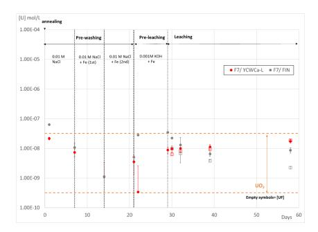
**Figure 2.1.1.5:** Second type of experiments - U concentration as function of time with F7 pellet for the autoclave experiment with Pt/Pd catalyst under  $H_2$  atmosphere at pH 13.5 in young cementitious water (YCWCa-L) and pH 8.5 in bicarbonate water (FIN).
