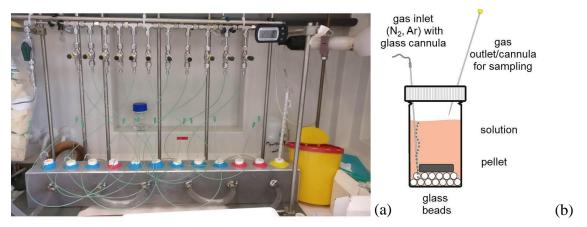
Figure 2.1.2.1: (a) Experimental setup of the dissolution experiments. (b) Schematic draw...<sub>8</sub> of the experimental vessels for the accelerated dissolution experiments.
