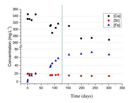
Figure 2.2.1.2: Evolution of the water chemistry as a function of time. The MOX pellets were introduced after three months of corrosion of the iron foil (vertical line).
